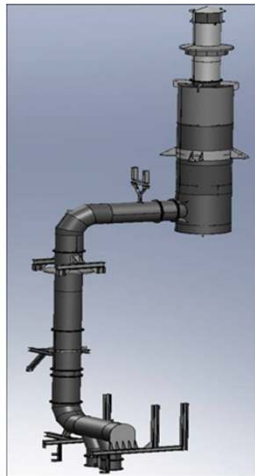
Exhaust system and air intake system with filtration for nuclear application diesel engine
